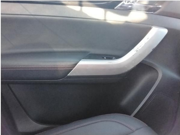
10: Door Pad nsr Scuffed Over 25mm
