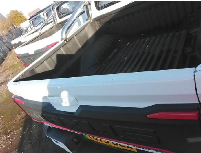
5: Tailgate Dented With Paint Damage
