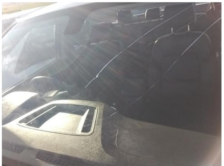
8: Screen Front Cracked Replace
