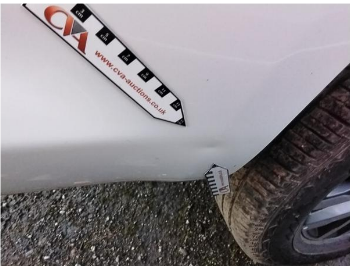
7: Qtr Panel osr Dented Over 30mm
