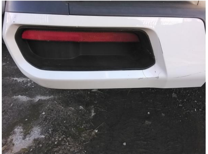
4: Bumper Rear Moulding Broken Replace
