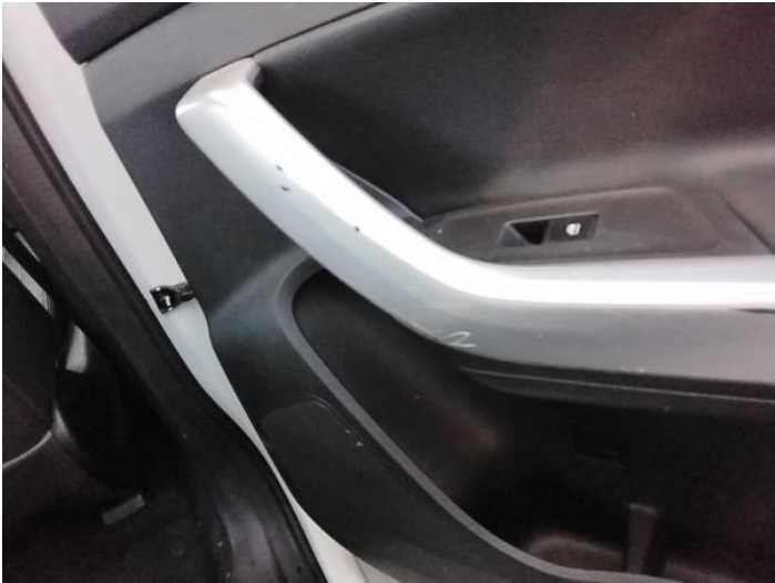
9: Door Pad osr Scuffed Over 25mm
