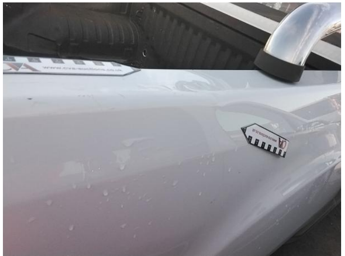
6: Qtr Panel osr Dented Over 30mm
