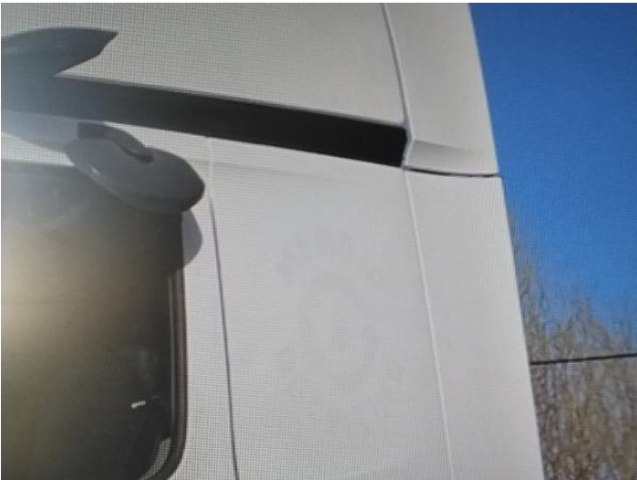
1: Wing nsf Scratched UpTo 25mm Thru Paint
