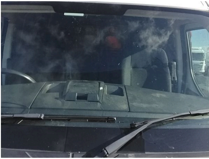
3: Screen Front Chipped Over 10mm
