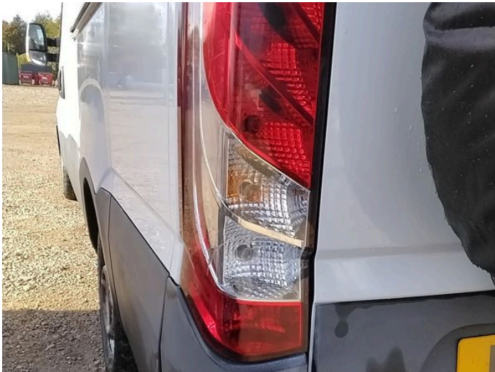
7: Lamp nsr Broken Replace
